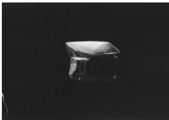
Figure 1 A photograph of a TS-Phy crystal. The crystal size is 0.4 × 0.4 × 0.5 mm. Although the surfaces of the crystal are rough, it is a single crystal.
